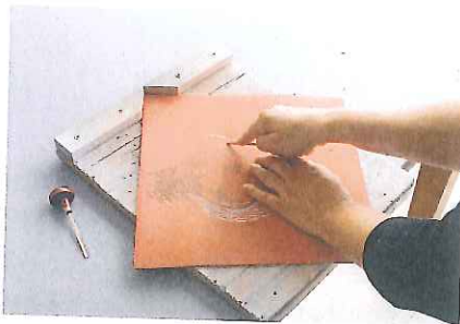
⌚ The pressure of cutting pushes the bench hook up against the table and pushes the block up against a second stop on the bench hook. A notch in this second stop allows the block to be turned at an angle as well.
