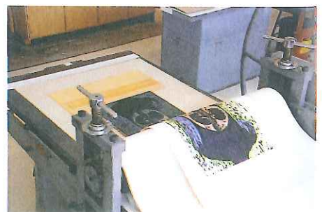
5–6. The second layer block is removed and replaced with the final key block to generate the composite image.
