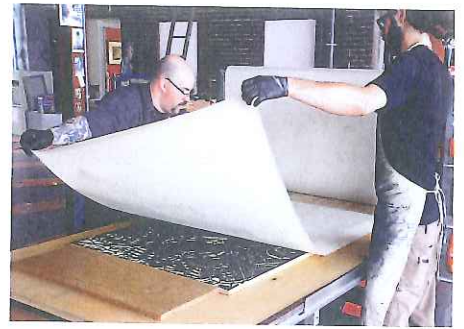
3. The paper is placed using a T and bar registration (located on running boards).
