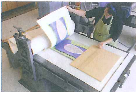
4. The second layer here is comprised of a set of jigsaw pieces which have been inked in three different colors. The outer shapes have been wiped so that just a halo of green ink remains.
