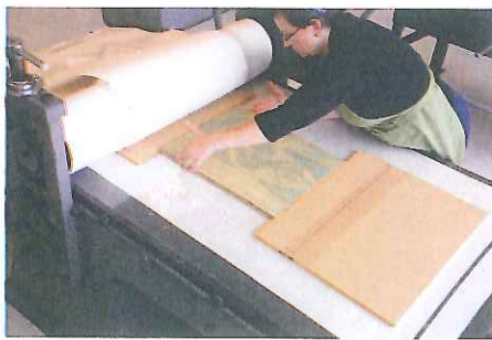
1. The paper has been engaged under the roller and the first block is placed in position.
