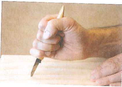
⌚ Almost all cutting is done by pulling the knife toward the cutter. It is not necessary to cut very deep, and, the finer the detail, the less depth is required.
